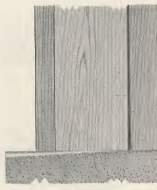
Side Jamb Set on Stone Sill
